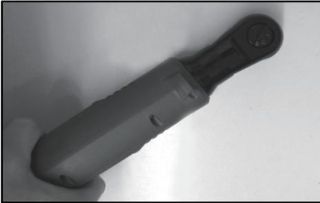
Hold the tool firmly and place the socket over the bolt/nut. Turn the tool on and fasten. When the bolt/ nut reaches the seating position, the tool stops automatically.
