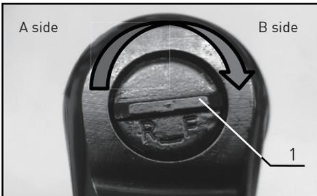
This tool has a reversing lever to change the direction of rotation. Turn the reversing lever to the A side for clockwise rotation or to the B side for counterclockwise rotation. Make sure that the reversing lever is fully turned with a click.
